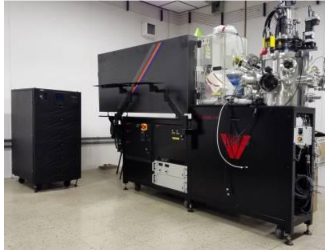
Pulse Laser Deposition (PLD)/ MBE - equipado com RHEED
